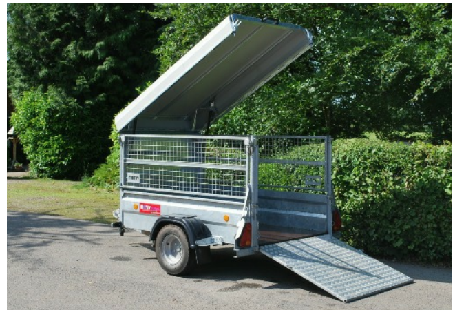
Relo 64 with mesh side gates, stock lid with gas struts and ramp tail gate.
