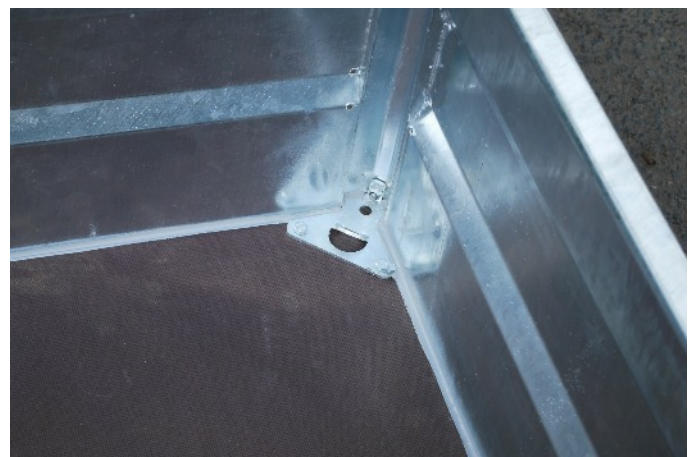
Standard internal lashing points.
